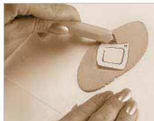
Use a sharp edge to cut BRONZclay™.
