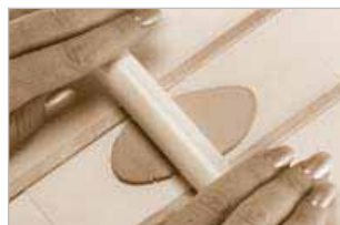
Use stirring sticks as a thickness gauge.
